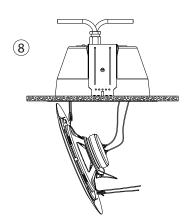
Fitting the speaker. Compress "V" spring and fit into the retaining ear within the dome. Connect leads to the speaker transformer. 9
