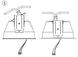
Re-fit plate to dome and tighten the wingnut
