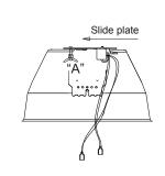
Loosen wing nut "A" (do NOT remove the wing nut completely) If the wing nut is on e .g. your left, slide the whole plate to the left.
