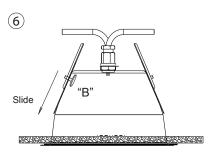
Fitting the dome into a ceiling Loosen the retaining knob for slider "C" Push sliders to the top of the dome and insert dome into pre-cut hole.
