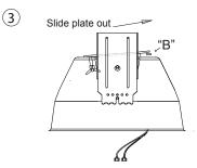
Lift the disengaged plates "B" side slightly and slide the plate out of the dome.
